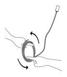
Very carefully uncoil the braided coaxial cable in a spool like
